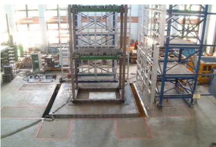
3D earthquake simulator (5m x 5m)
