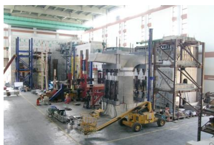
L-shape reaction wall and strong floor
