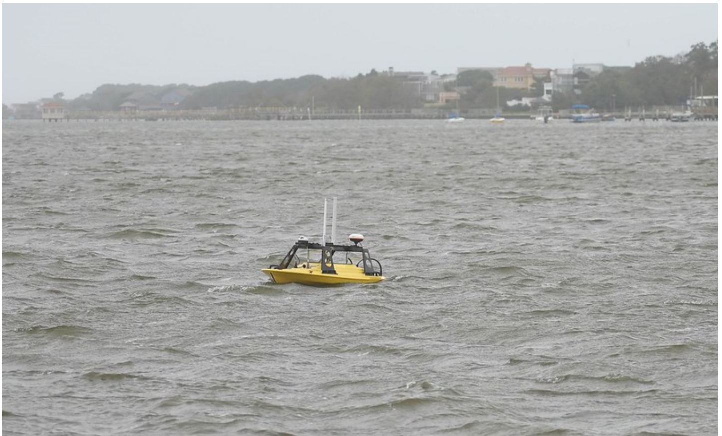
The RAPID hydrographic survey vessel. (Photo: A. Renaud)
