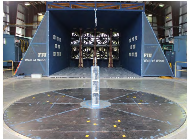
Aerodynamic wind testing at the NHERI FIU WOW to obtain wind pressure time histories distributed on the building.
