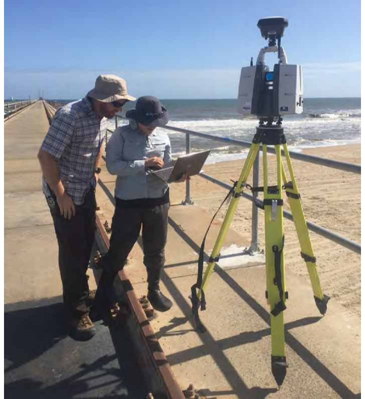
RAPID Operations Manager Michael Grilliot and Operations Specialist Jacqueline Peltier laser scan waves off a pier in Duck, North Carolina. (Photo: RAPID Facility)
